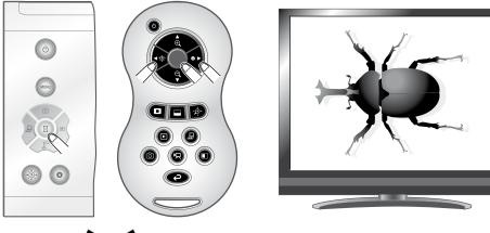
In this status, press the [ ] button on the remote control to display another image in the thumbnail list.
