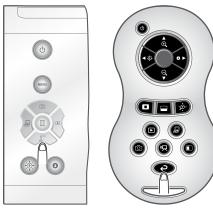
2 Make sure that the menu is not displayed on the screen and press the [ 2] button on the operating panel or the [ 2] button on the remote control.
