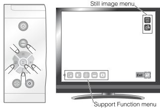
Move the cursor using the [ ] button on the operating panel and select a menu item with the [ ] button.
