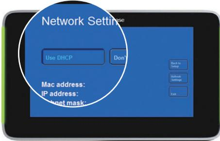
DHCP must provide an IP address, gateway, and domain name or the RoomWizard will reject the DHCP settings. If the RoomWizard rejects the DHCP settings, it will adopt a default static address. You can use this default or another static address to access the RoomWizard’s web-based setup pages and enter DHCP settings manually.
